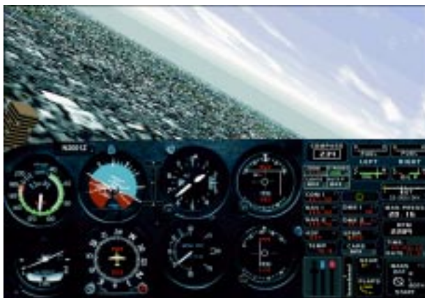
Turn onto downwind heading 180 degrees, 120 knots, 1000 ft AGL. Power setting should be around 2300. Note the 30 degree angle of bank.
